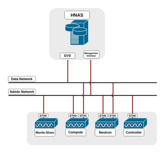
In Neutron Node, create a bridge (e.g. br-hnas) and add the data interface to this bridge:
