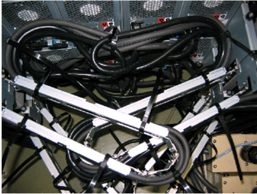
Figure 5-38: ENC Cable Routing on High-density Expansion Unit
