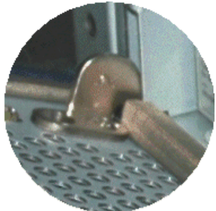
Figure 5-49: Installing a Front Bezel
