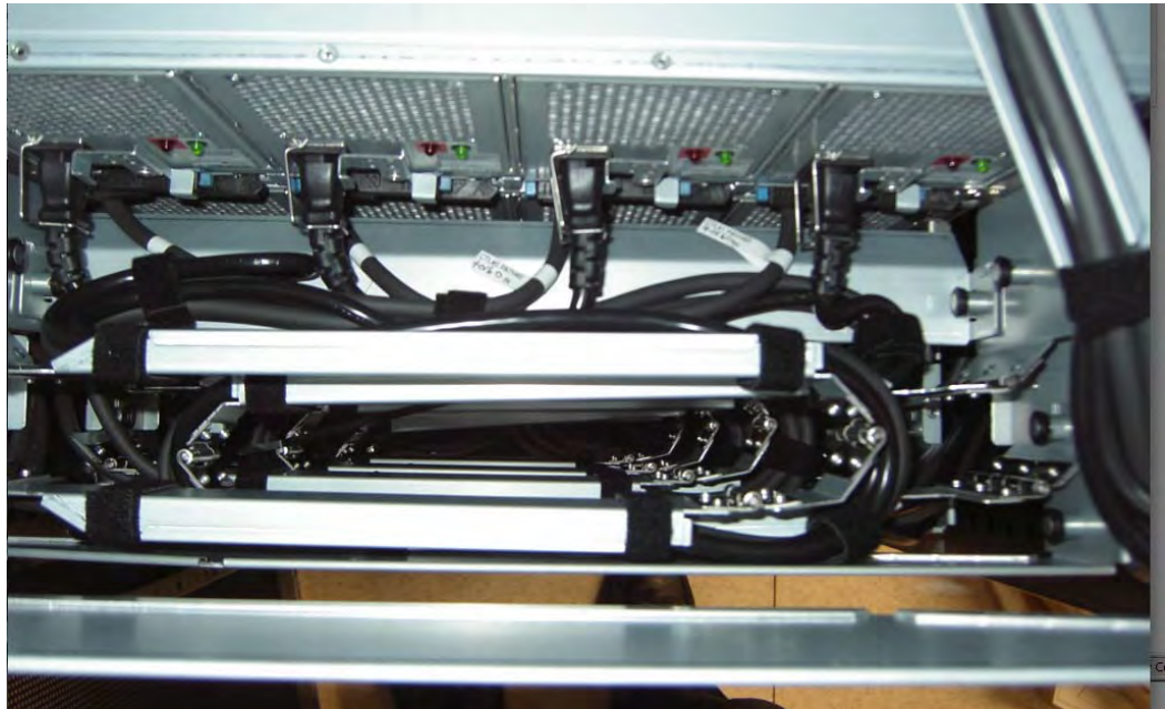
Figure 5-2: Cable Guides (Vertical View Looking Down)
