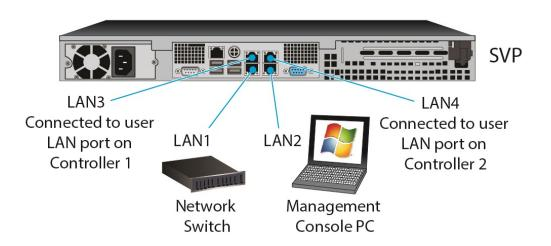
After you connect the physical SVP, you can set up an encrypted Secure Sockets Layer (SSL) connection between the storage system and the SVP.
